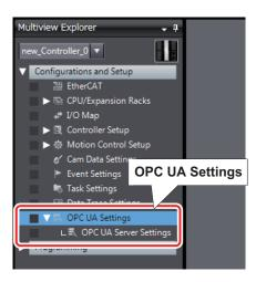
There are three types of **OPC UA Settings**; items that are recorded in the project file in the Sysmac Studio, items that are not recorded in the project file in the Sysmac Studio and required to be set for each CPU Unit, and items that are only displayed or operated without any setting. The differences of each are described in the table below.
