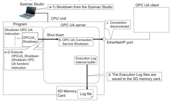
a. The OPC UA Server is shut down by one of the followings: (1) Using the Sysmac Studio Or(2) Executing the OPCUA\_Shutdown (Shutdown OPC UA Function) instruction
