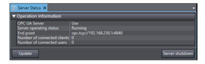
You can check the following states unless the operating status of the OPC UA Server is *Initializing* or *Shutdown*.
