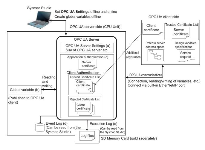
**Note** The above figure shows the case of a self-signed client certificate.
